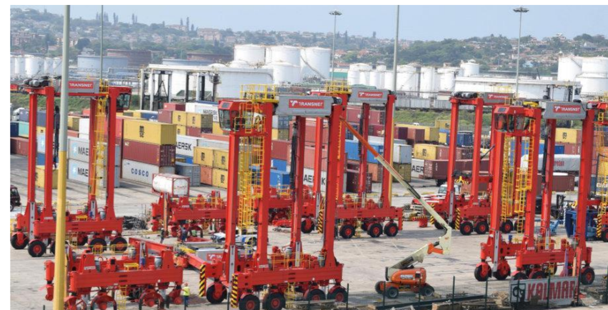
Durban Container Terminal's straddle carriers
